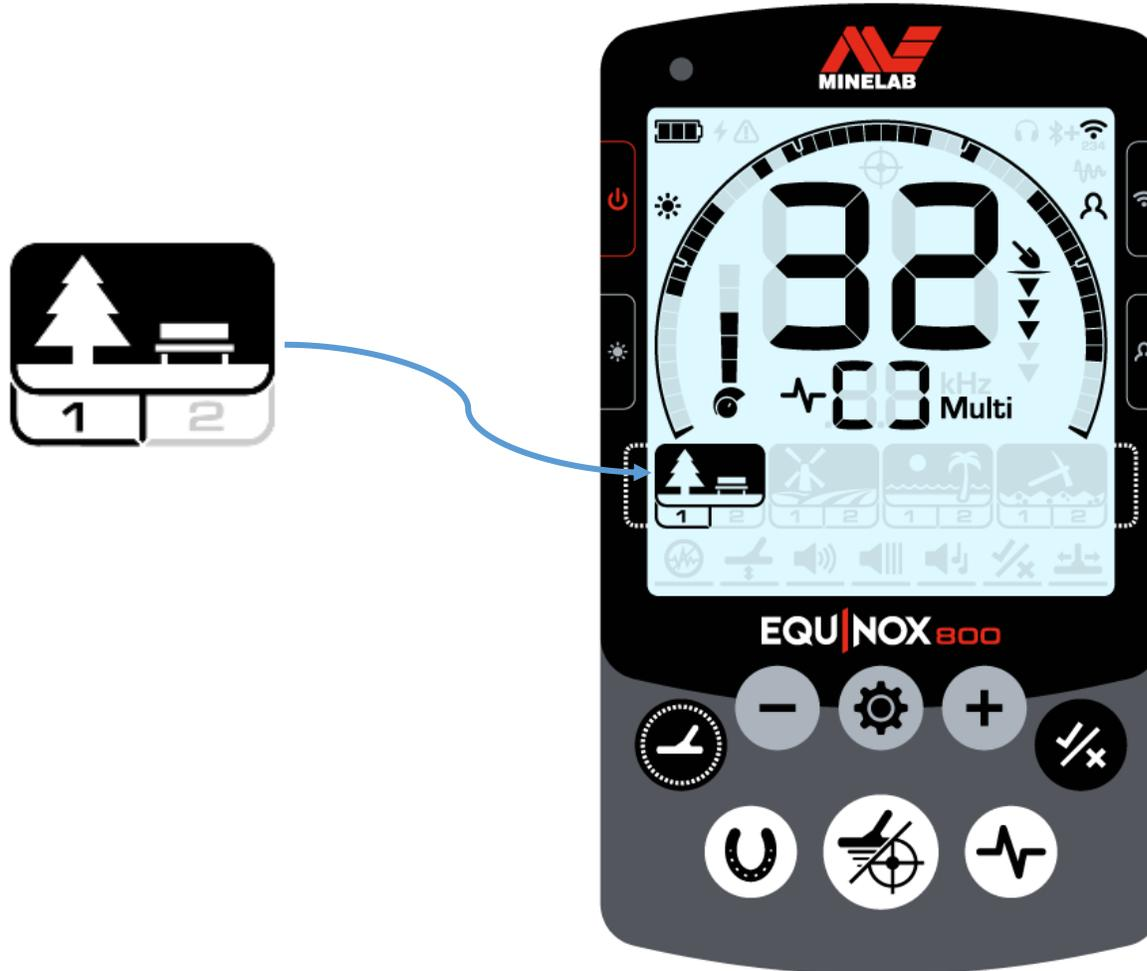
For each Detect Mode, the default Search Profile 1 setting has been optimised for easy detection of a wide range of targets.
