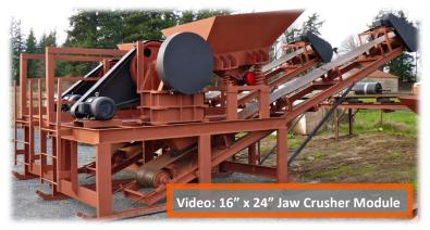
Turn-key jaw crusher system, powered with three phase electric motors
